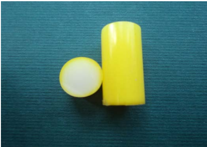
UHMWPE sample after the treatment by sc-CO 2 with a dye "Sudan Yellow"
